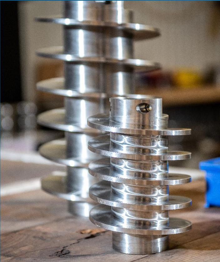
The auger draws the product into the milling chamber.
