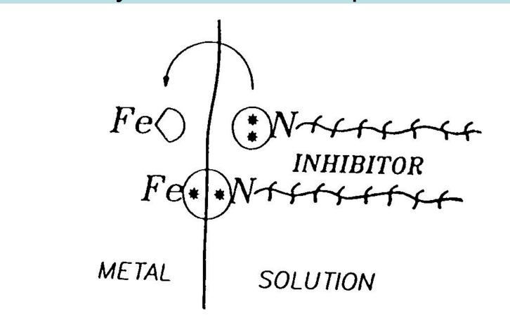
Creation of a chemical barrier at molecular scale
