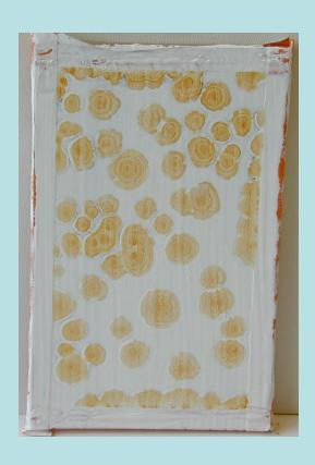
Properties deterioration : adhesion loss, permeability increase
